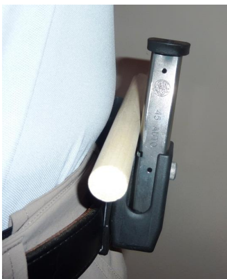
Ex. 8.6.1.5 Not Legal fails dowel test and 8.6.2.6 has knob extending past outer face
